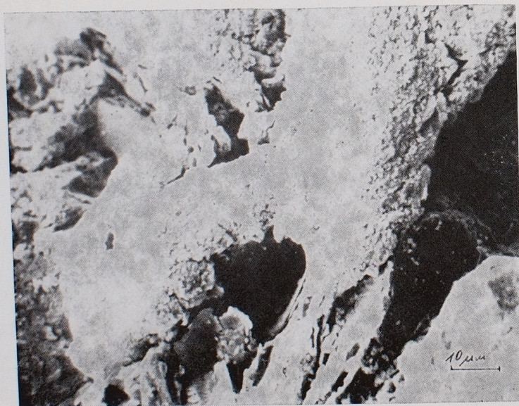
Phot. 4. Surface of a quartz grain from kaolinite zone of kaolin crust in Bolesławice. Electron scanning microscope. \times 1000
